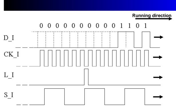
Description: There is a "gradual change" mode in HL1606, so D\_I only need one set of data"10110000", then input "0" to the end is okay. Clock signal has been sent to CK\_I, sent a "1" to L\_I after 8 clock signal. Change once the signal of S\_I, the output decline in a series. A clock cycle in S\_I, output is keep in 512Hz refresh frequency, to maintain the same level(series) of output duty cycle refresh. If no data sent to S\_I,
